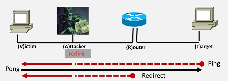
Bypasses "secure redirect" check, default on all OS. IPv4: remote, IPv6: local only
