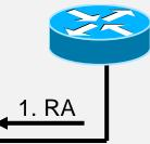
ICMP Type = 134 Src = Router Link-local Address Dst = FF02::1 Data= options, prefix, lifetime, <u>autoconfig</u> flag
